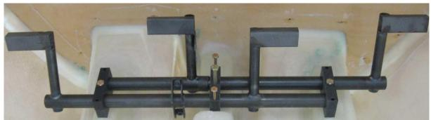
Fit the rudder pedals into place as shown above, with the mount blocks supporting the pedal assembly. Check each lower block to see if it is touching both the floor mounts and the rudder pedal assembly main bar. If any block can be moved up and down then you should follow this procedure, otherwise skip this task and go to the next task.
