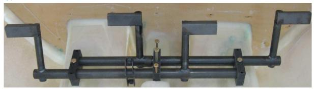
Now fit the top of the mount blocks: working on one mount block at a time, remove the centre bolt, place the top of the mount block in place and replace the centre bolt. Place all three bolts in the centre mount block and do them up by hand until the bolts reach the bottom of the captive nuts – this will ensure that no flock will get into the threads. Carefully rotate the rudder pedal shafts by moving the rudder pedals forwards and backwards – there should be no binding whatsoever.
