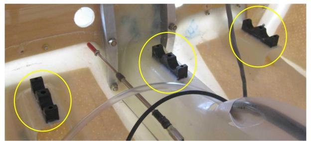
Smooth off any excess flock with a small amount of resin on a clean mixing stick. Leave to cure, taking care that no flock has contacted the rudder pedals. When the flock has gone off and is firm, carefully remove the bolts. Once the flock is completely cured remove the top of each mount block and the rudder pedals and set them aside until after the paint and upholstery tasks have been completed.
