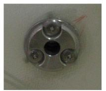
Screw the left-hand *pivot bush* firmly into the *pivot barrel*. Push the pivot barrel through the console and flock into place then loosely fit the right-hand side pivot bush. Line up the left-hand side rivet holes and secure the left-hand side *pivot bush* with three TLR rivets as shown at left.
