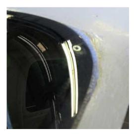
When you are satisfied that the windscreen is positioned correctly wipe away the excess flock with a clean mixing stick, taking care not to smear any resin or flock over the windscreen: always wipe out and away from the windscreen. Do not use any cleaning agents; use only a clean soft cloth.
