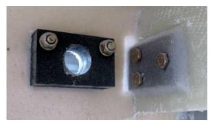
Next day tighten the Nyloc nuts firmly and do a final check for binding, then remove the flap drive shaft completely: pull it out through one side of the fuselage, clean off the wax, make sure that the inner and outer shafts are fitted together then reassemble the drive fittings to the shaft and store for later use.
