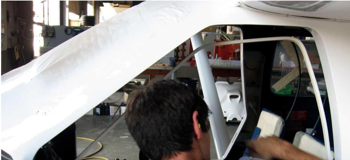
Unscrew the top and front of the top sections of the door jamb – leave the rear of the jamb screwed in place to keep the alignment. Slide the gutter in place between the fuselage and the jamb and push it in so that there is the absolute minimum of gutter exposed to the airflow.
