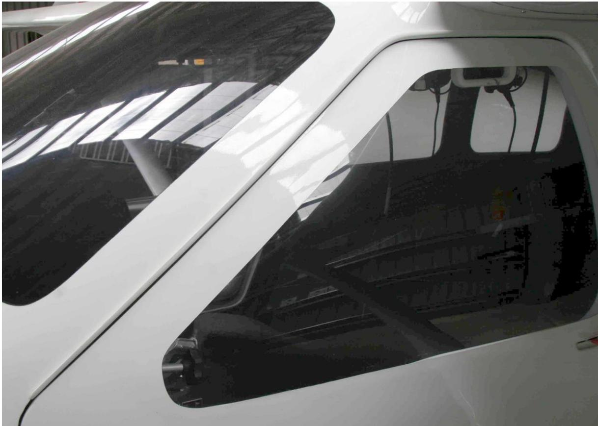
The photo above shows a completed gutter. Note that the gutter only protrudes very slightly outside the fuselage. Note also that the fuselage, doors and gutters are all painted separately prior to the gutter being final fitted.
