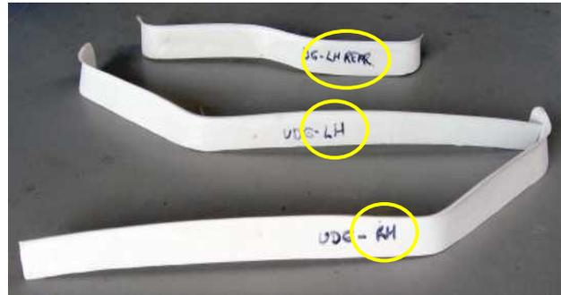
The gutters are not painted: in the case of a **normal build** the gutters will be pre-fitted and the doors adjusted in *Pre-paint* and then the gutters will be painted and finally fitted later as part of the normal build sequence.
