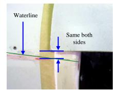
centred at the front and back, mark the centreline on the cowl and on the fuselage in front of the windscreen and then tape the cowl to the fuselage.
