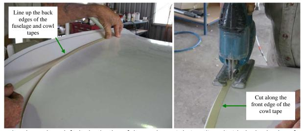
In the photo above left the back edge of the cowl tape is being aligned with the back edge of the fuselage tape, while in the photo above right the cut is being made in line with the front edge of the cowl tape. Sand any rough edges away with a long sanding block and refit the top cowl, using the centreline mark to position the cowl at the back and checking that the front of the cowl is still centred, then tape the top cowl into place.
