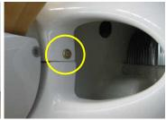
remove one 6G stainless steel screw at a time and drill the hole out to 3/16", then drill the 3 holes in the top cowl to 5/16".
