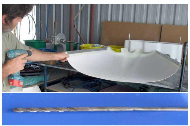
Next day test fit the hinge pins and remove any remaining flock from the hinges. In the factory we use a special drill bit (shown above) that is just a standard drill bit welded onto the end of a spare hinge pin and we clean the hinges through with that (top photo), using a low drilling speed to prevent any whipping of the long bit. It is important that the hinge pins fit easily into the hinges without any restrictions.
