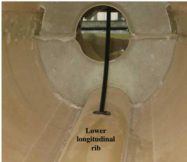
Keep feeding it in until it can be seen near the rudder slot on the left-hand side of the lower console as shown at lower right, then use a hook to pull it through the slot and pull it about 150mm through and into the cabin footwell.
