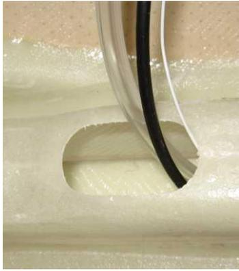
When the bundle is visible in the cable hole at the lower front of the console pull it through until the cloth tape can be removed, then withdraw the elevator cable from the rear while holding the electrical cables and the static tube from moving back – tape them to the side of the console if necessary.
