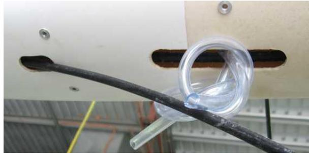
The VHF antenna cable and any tail strobe wiring can be left trailing out the rear of the fuselage at this point – they will later be routed up and into the vertical fin. The 2 fuel pump wires can be pulled up through the hole in the lower longitudinal rib behind the rear bulkhead along with any wingtip strobe wiring for later connection.
