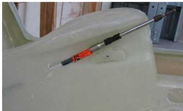
Clamp the elevator cable into place using the supplied clamp bracket, taking care to fit the pressed locating section of the clamp in the groove around the outer cable. The clamp consists of a saddle and a backing plate, and the whole clamp must be fitted onto a tapered profile plate with the thin end of the wedge facing the rear of the aircraft and secured to the fuselage by 2 x AN3-6A bolts and Nyloc nuts. Tighten firmly.
