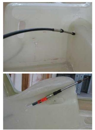
Clamp the elevator cable into place using the supplied clamp bracket, taking care to fit the pressed locating section of the clamp in the groove around the outer cable. The clamp consists of a saddle and a backing plate, and the whole clamp must be fitted onto a tapered profile plate with the thin end of the wedge facing the rear of the aircraft and secured to the fuselage by 2 x AN3-6A bolts and Nyloc nuts. Tighten firmly.
