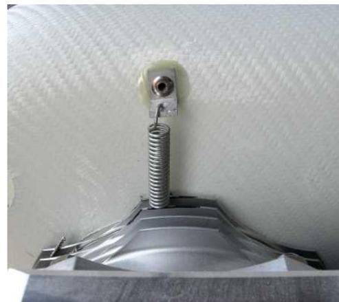
Fit a loop of lock wire around the cylinder between the third and fourth fin and through the bottom of the spring and twist it off.
