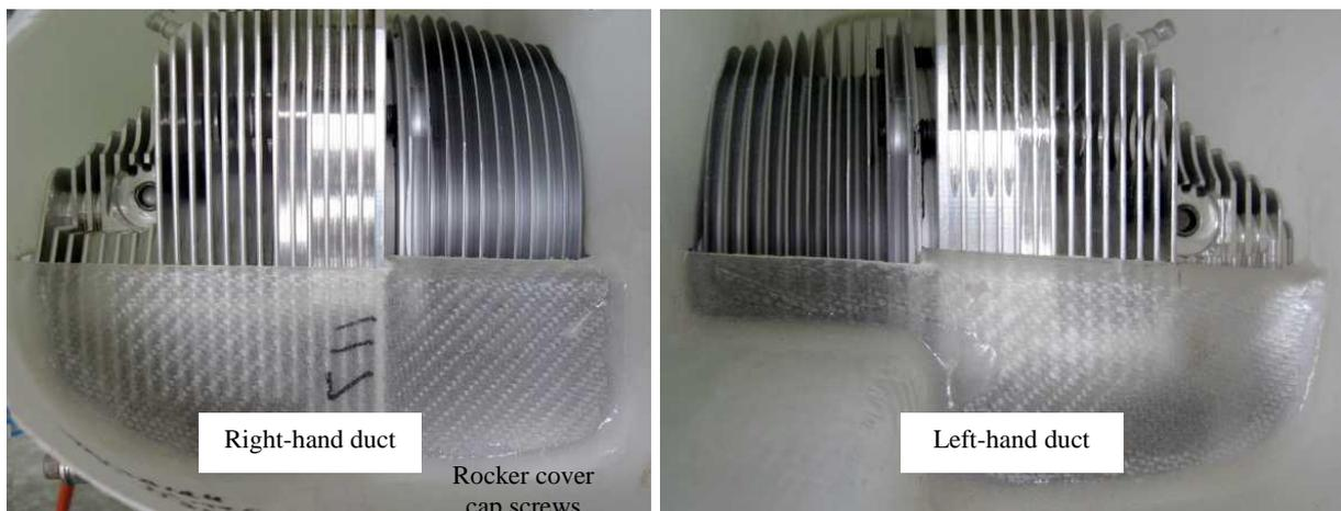
The front air dams will need to be trimmed to fit around the fins on the cylinder heads and barrels. The final fit must have the air dams only just touching the fins as shown above.
