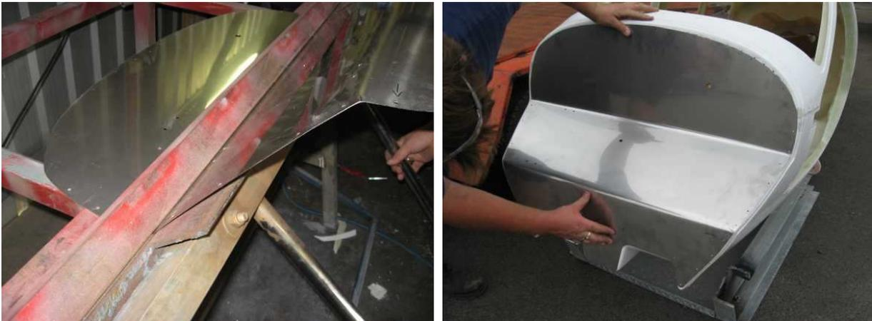
These photos show the upper bend being made and the plate sitting in place. In our factory the bending process takes a skilled person about 15 minutes – it is not a complicated task so long as you take care to measure accurately and bend carefully and in the correct sense.
