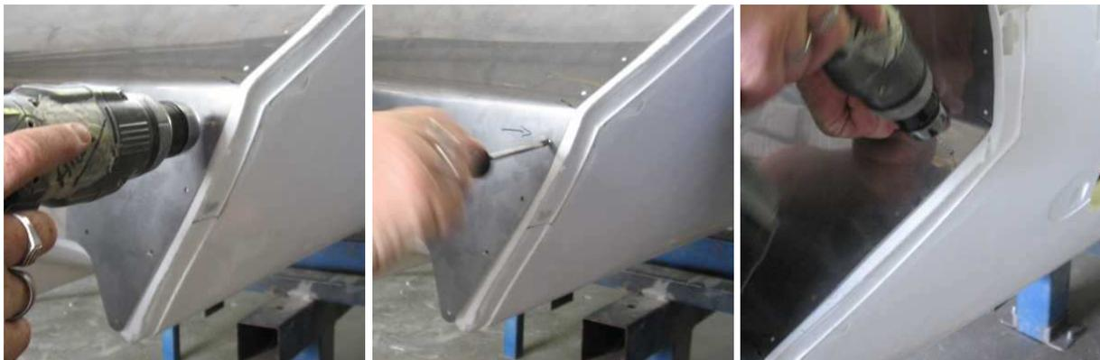
Apply the Dow Corning silicone sealant to the back of the firewall plate in the same manner: around the outside and across the rest of the back, then place the plate onto the insulating sheet and push firmly into place using the lower part of the firewall sheet as a reference. Secure temporarily with 2 self-tapping screws at the base of the upper bend on both sides and 2 more in the holes just below the upper bend.
