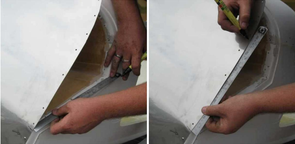
Measure from the centre of the lower bend back to the centre of the upper bend on the fuselage and transfer that measurement to the firewall plate – note that the measurement may be slightly different from side to side so measure each side independently. Recheck your measurements and then remove the plate, transfer the lower bend marks to the back of the plate and take the plate to the bender.
