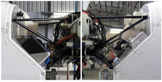
Attach the engine mount to the firewall with the top (AN4-20A) bolts only: fit each bolt from the front, through the mount, firewall, and the backing plate (shown at right) and fit a washer and Nyloc nut.
