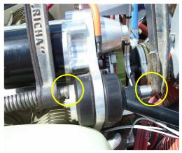
the steel lock nut, as shown at right. The clamping points have been circled in yellow.
