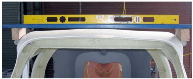
**Lateral plane**: place a 3" block on the top of each front wing mounting lug and place a spirit level or a digital protractor across the top of the cabin so that it rests on both blocks. Pack the main wheels as required to level the aircraft.
