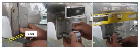
Place a straightedge or ruler under the centre of the fuselage and measure up 5mm. This is the position for the bottom of the square outer backing plate for the nose gear housing.
