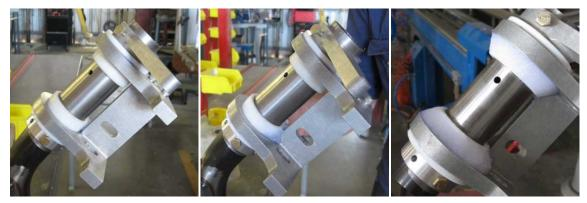
Fit the assembly onto the nose leg with a retaining collar or yoke bolted to the top and check for freedom of movement. When you are satisfied that there is no binding, mix a small batch of flock and flock the bushes into the plates, taking care not to get any flock onto the nose leg.
