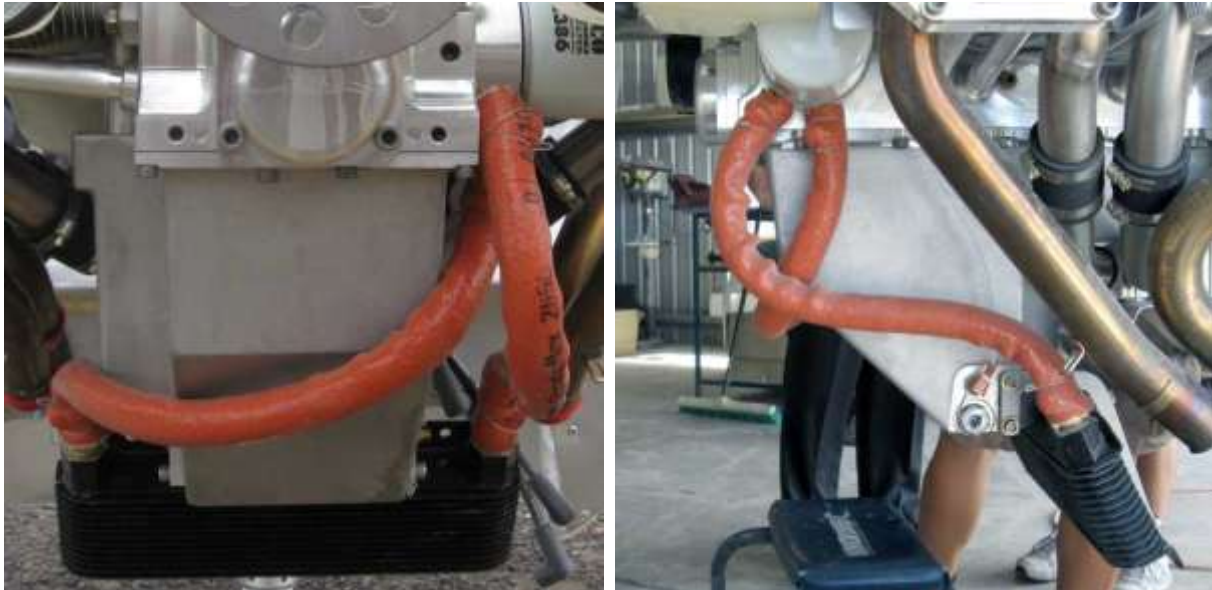
Completed oil line arrangement between the adaptor and the oil cooler
