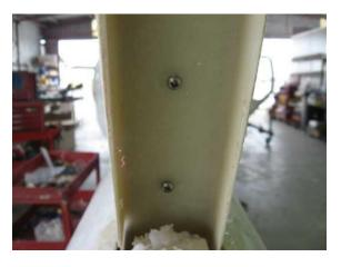
and the rudder cable and remove the self-tapping screws. **Recheck the vertical alignment**. Wax one side of each of 2 lengths of aluminium channel so that the flock will not stick and place as a rail along each side the full length of the join line and secure with clamps as shown below. **Recheck the vertical alignment**. Leave overnight to cure.
