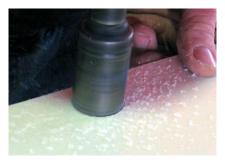
Start by laying the vertical fin on its side and drilling out the marked inspection hole on the left-hand side with a hole saw.
