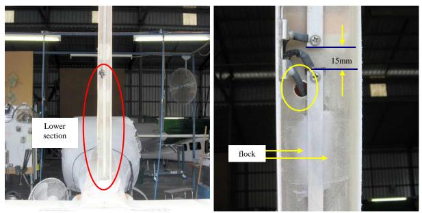
Ensure that the VHF coax cable exit hole is on the hinge (left-hand) side of the vertical fin – elongate the hole with a file if it is not. Sand the back of the lower section of the VHF antenna and place it so that it is exactly 15mm below the upper section and fix it in place with 5-minute Araldite.
