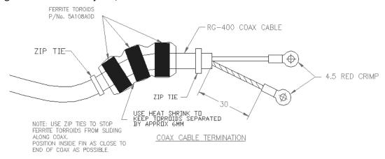
Screw the inner cable to the TOP section and the braided coax sheath to the LOWER section. Tuck any excess cable back into the vertical fin and seal completely with silicone sealant.
