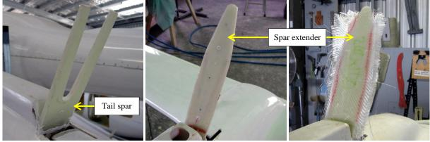
Sand the matching surfaces of the pre-fitted tail spar and the spar extender. Make sure that the 2 pieces match and then fix the spar extender in place with 5-Minute Araldite.
