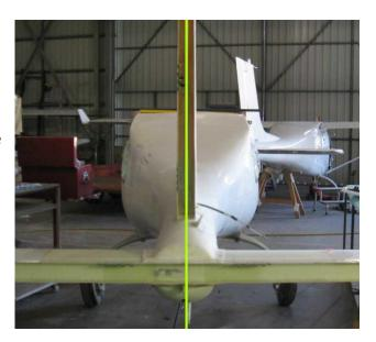
the fin when viewed from the rear. **Recheck this vertical alignment** at every step from here on.
