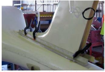
Next day remove the aluminium channels and the peel cloth, then use a hole saw to open the inspection hole and a drill and jigsaw to recut the rudder cable slot. File out any rough edges.
