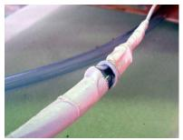
Pull the static tube/strobe wiring and the VHF cable through the fin and out of their respective holes, then tie a knot or tape a mixing stick across the end at right angles to prevent them sliding back inside the fin.
