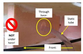
Tie the drawstring to the VHF cable and the draw wire to the static tube/strobe wiring. The photos below show how: loop the draw string or wire around the cable or tube to be pulled then tape the end of the draw wire or string so that when it is pulled it will tighten the knot. Tape the end of the cable or tube to be pulled to streamline it and avoid it catching on anything. Cloth tape is stronger than masking tape and is recommended for this purpose.
