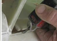
Check the fit along the entire joining line and mark and remove as required to achieve a good fit. Take extra care to ensure that the join at the front of the strake (at the yellow arrow in the photo below) is smooth so that there is one continuous line along the entire length of the strake – if there is any discontinuity it will look extremely disappointing when paint is applied so take care to get it exactly right at this time.
