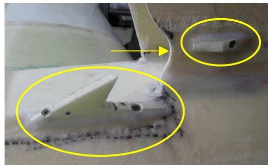
It may also be necessary to sand away part of the lower right of the fin (arrowed at right) to allow clearance for the rudder arm at full right rudder deflection.
