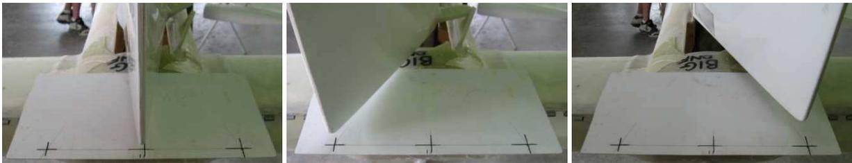
Make a template that will sit over the rear of the empennage and tape it in place. Find the centreline of the fuselage and mark a 5mm offset to the right onto the template, then mark 100mm each side of the offset as shown above. Refit the rudder.
