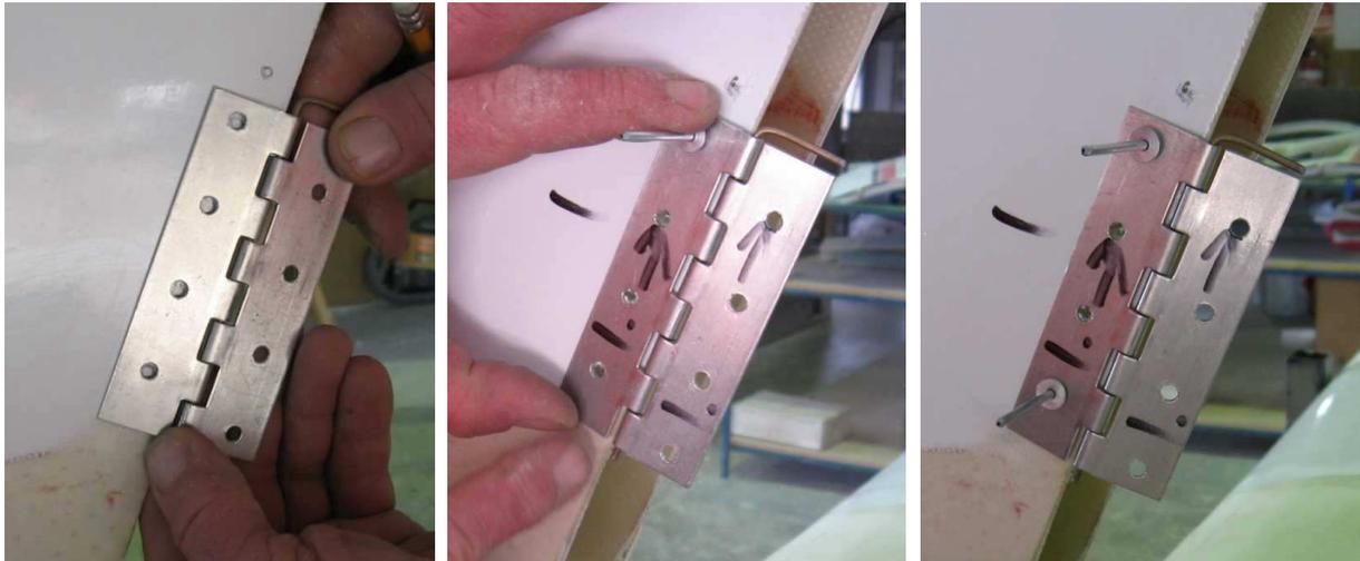
Hold a hinge in position and drill the top hole only and temporarily fit the hinge in place with a rivet as shown above, then carefully reposition the hinge so that the hinge pin is parallel to the back of the rudder and drill the bottom hole and fit a rivet in that hole, then drill the remaining 2 holes. Repeat this process for each hinge.
