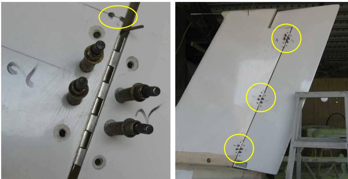
Test fit the rudder using Clecoes to hold each hinge in the final mounting position, which is inside the fin and inside the rudder as shown above. Remove the spacers and check that the rudder can swing freely left and right at least 100mm from the centreline as measured at the rear of the rudder. If there is any binding locate the source and correct it.
