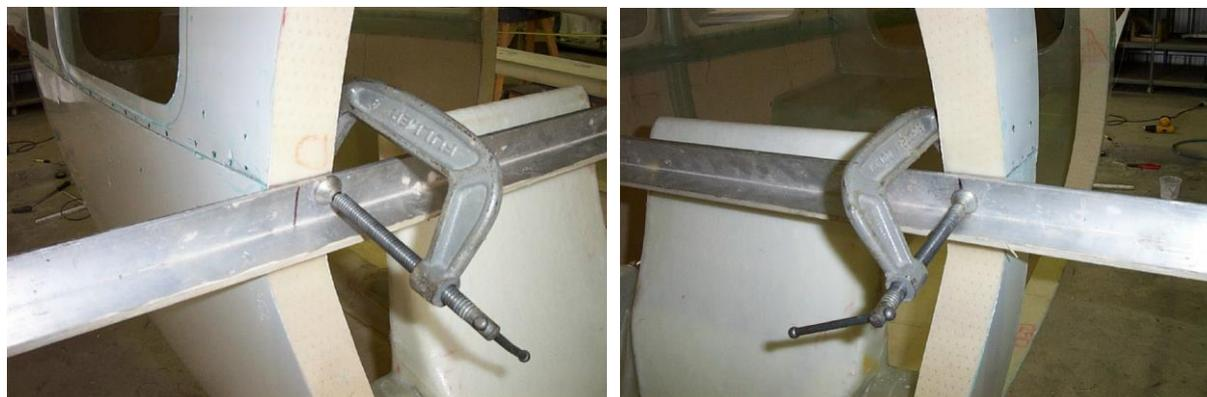
Clamp a straightedge (a 2 or 3 metre length of aluminium angle works well) across the back of the door frames at the height of the fuselage join line: ensure that the straightedge is level. This will be your main reference for aligning the horizontal stabiliser.
