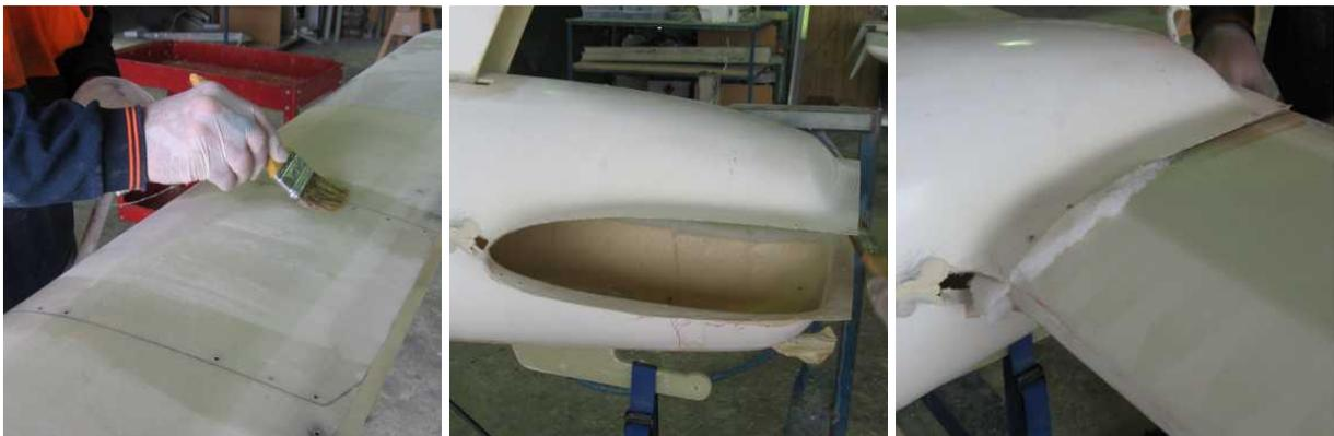
Mix a batch of resin and divide into 2 parts. Coat all the surfaces to be joined. Add flock to one part of the resin and apply a layer to the rear of the fuselage then slide the stabiliser in to place, pushing it fully forward. Open the joint and use a mixing stick to force flock into the sides and rear of the joint, then smooth the flock along the outside. Fix the stabiliser in place with the self-tapping screws, do a final check of the alignment and leave overnight to cure.
