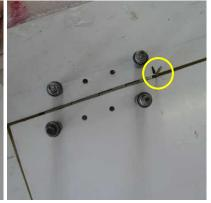
Test fit the hinges using 2 Clecoes per side and slide the hinge pin into place as shown above. Fit the 2 outer hinges first – this will hold the elevator in place while the inner hinges are fitted.
