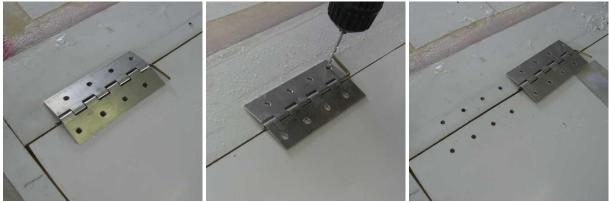
Use a 3/32" drill to make a pilot hole opposite the pin side of each rivet hole: this is to allow for the slight slope of the hinge at this point, then check that the hinge and hole positioning is correct and then carefully expand to 3/16" holes.
