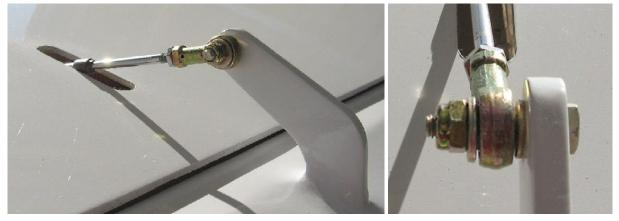
Fit the aileron cable rod end to the aileron drive arm with an AN3 bolt fitted through the drive arm, then an AN960-416 (3/16") flat washer, then the rod end followed by an AN960-515 (1/4") flat washer and a Nyloc nut as shown in the photos above.
