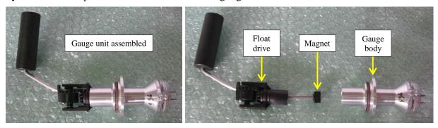
The gauge can then be reassembled and rechecked (and readjusted if necessary) until it reads correctly.
