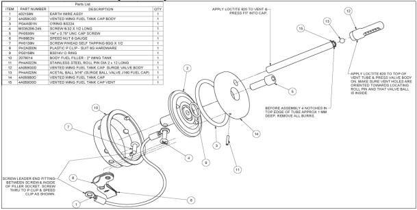
Use a file to cut 4 notches each 1mm deep into the top of the vent tube. Remove all burrs.
