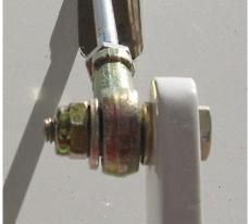
Fit the aileron cable rod end to the aileron drive arm with an AN3 bolt fitted through the drive arm, then an AN960-416 (3/16") flat washer, then the rod end followed by an AN960-515 (1/4") flat washer and a Nyloc nut as shown in the photos above.
