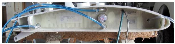
There are 3 fuel lines that need to be connected in the wing root: the bottom 2 carry fuel to the header tank while the top line is the breather for the header tank. These fuel lines were cut to the approximate length in the *Pre-Paint>Fuselage>Interior>Fuel System* task and stored until now.
