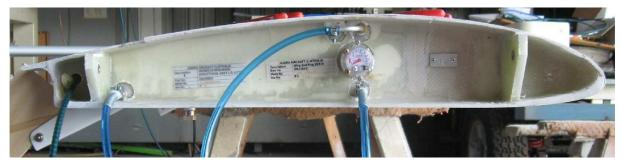
There are 3 fuel lines that need to be connected in the wing root: the bottom 2 carry fuel to the header tank while the top line is the breather for the header tank. These fuel lines each need to be fitted and then cut to an approximate length of 300mm behind the rear of the wing.
