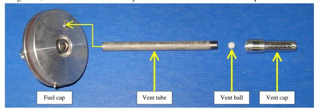
Working on one wing at a time, remove the fuel cap and place a clean cloth or a piece of tape over the fuel filler opening so that no dirt or debris can fall into the tank during this process. Start by carefully cleaning away any paint from the top of the fuel cap and in particular from the vent tube hole in the top of the cap.
