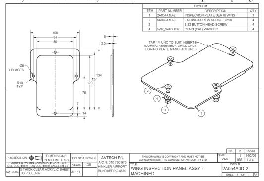
Fit the threaded fairing sockets to the inspection cover and then position the cover inside the wing and fix in place with 8-32 button head screws, all as shown in the drawing above.
