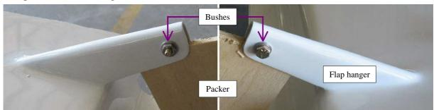
Keep the flock away from the bolt holes, fit a flap pivot bolt though the bushes and then fit and tighten a plain nut just enough to hold the bushes firmly in place. A packer should be used to avoid the flap hanger flexing in when the bolt is tightened. Smooth the flock carefully with a clean mixing stick dipped in resin and leave overnight to cure.
