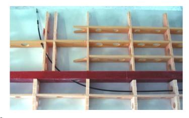
It will help if your helper can slowly rotate the outer cable while you ease the cable around the curve at the outboard end of the wing. Do **not** pull strongly on the drawstring: if you do you will only succeed in cutting the string into the foam ribs and wedging the cable, which will make it extremely difficult to complete the task.
