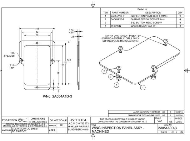
At this time you can fit the clear acrylic inspection cover to the inspection opening.
