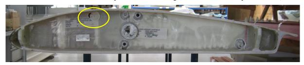
There is a drawstring inside in the wing with extra string coiled around a stick at the aileron end that will be visible through the aileron cable inspection opening. Loosen the drawstring and check that it can be moved freely, then pull a short length out of the wing root (circled above) and tie it firmly through the rod end. Wrap cloth tape around the cable end from the rod end all the way back to the outer cable: this will ease the cable through the wing ribs.
