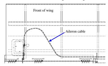
move the cable carefully and shake it if it seems to catch at any time.
