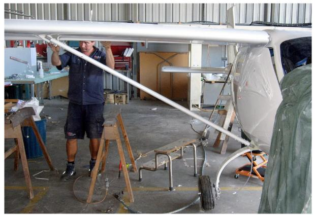
the strut to the wing with an AN175-15A bolt inserted from the front and an AN960-516 washer MS20365-528 nut and tighten up until the nut is in safety: there should be at least  $1\frac{1}{2}$  threads showing though the nut but not more than 3 threads showing.
