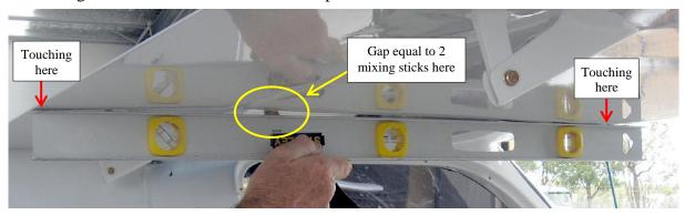
Hold a straightedge under the wing and flap with a gap equal to 2 mixing sticks at the rear of the wing and touching at the front and back, all as shown in the photo above.
