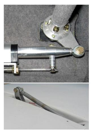
If you set your flap end clearances correctly in the *Pre-Paint>Wings>Test fit wings* task there should be no problems, but if the flaps do touch the fuselage then you will need to remove the flap and cut the end of the flap away to maintain a 5mm clearance from the fuselage.
