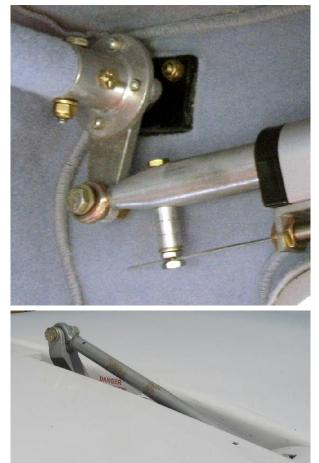
the *Pre-Paint>Wings>Test fit wings* task there should be no problems, but if the flaps do touch the fuselage then you will need to remove the flap and cut the end of the flap away to maintain a 5mm clearance from the fuselage.
