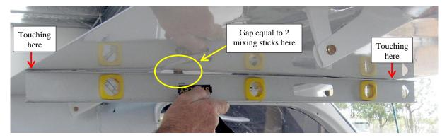
Hold a straightedge under the wing and flap with a gap equal to 2 mixing sticks at the rear of
