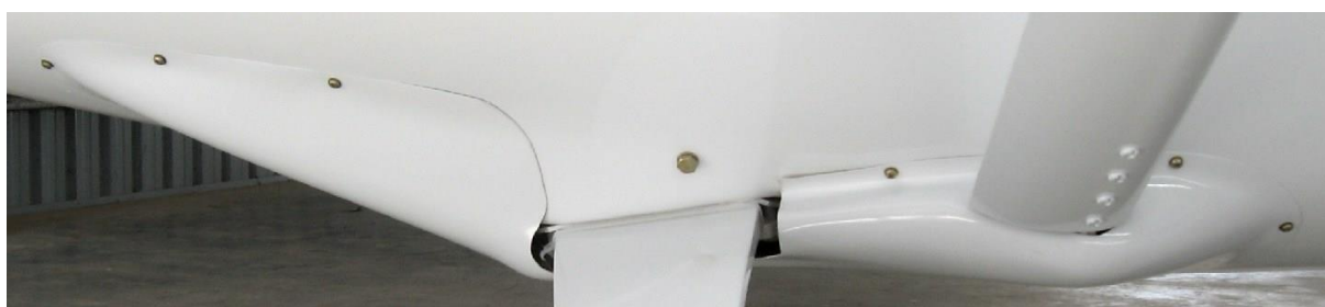
Right hand side strut/main gear fairing from below (top photo) and side on (above)
