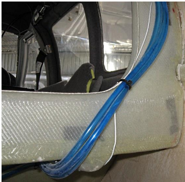
Example of fuel line routing behind the rear bulkhead.
