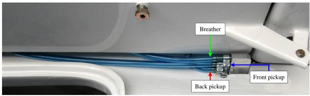
Hold the fuel lines under the connector block and cut each line to length so that they can be fitted to the connector block as shown above. There must be no kinks in any fuel line.
