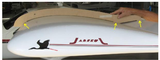
In the kit there is an aileron deflection template. Place this template on top of the wing and set the aileron to the full UP travel deflection as shown in the photo above (note the 3 arrowed points where the template touches) and then adjust the stop bolt on the aileron bellcrank so that the bolt just touches the eccentric stop at full deflection.
