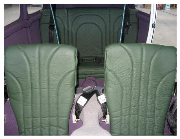
Identify the left and right side front seat covers. Slip each seat cover over the correct seat back and pull the cover as far down as you can, then roll the lower part of the cover over the seat base and pat the Velcro front edge into place.
