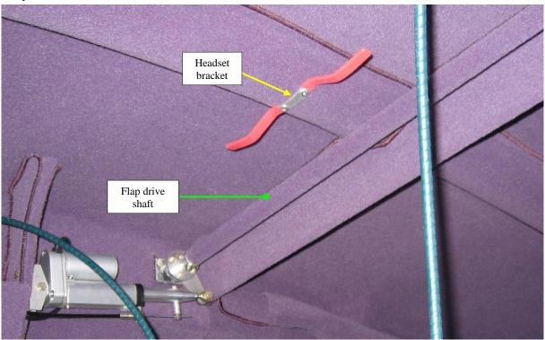
Wrap the flap drive shaft in upholstery fabric and fix into place with contact adhesive. The join line should be at the top rear of the shaft.
