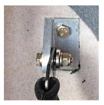
seatbelt fitting, then the heavy flat washer (from the "Seatbelts" card) and a plain washer then the Nyloc nut. Tighten the Nyloc nuts to safety.
