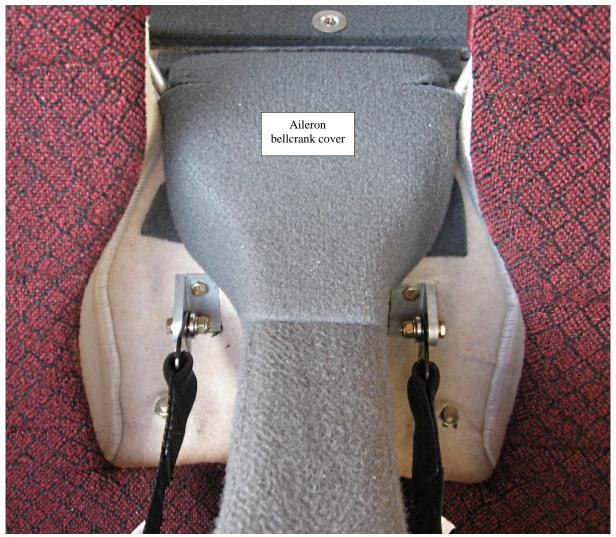
Bolt the seatbelts to the seatbelt fittings – the shoulder harness fits to the outside of each seat while the lap part of the harness fits beside the console.
