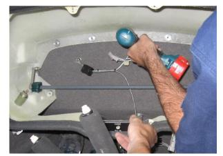
The drill bit will be visible as a point on the firewall before it breaks through and the person watching must be vigilant to prevent any possible damage. It may only be necessary to move a wire or something before drilling further.
