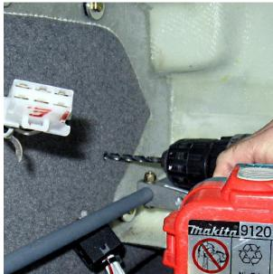
lever (which must face as shown) and then drill a pilot hole at that mark – rotate the throttle linkage backwards to allow access for the drill and hold the drill firmly against the firewall to make sure that it does not move about while drilling.
