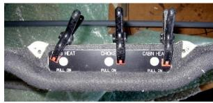
Drill out the 3 cable holes to suit the cable outer fittings.
