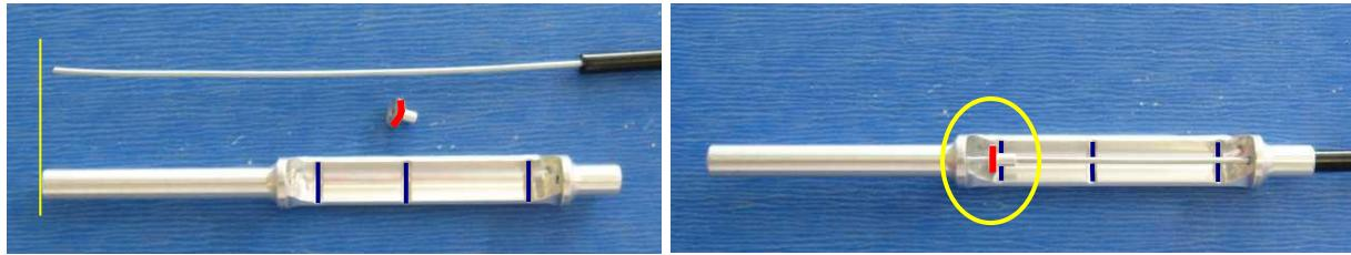
Assemble the flap indicator: paint the outside of the indicator washer red and mark the 3 flap positions in a dark colour. Push the inner cable through the indicator body and through the indicator washer then all the way into the long end of the indicator body.
