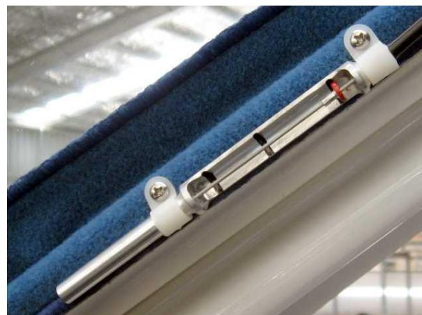
Check that all bolts and nuts are tightened, route the power lead behind the motor assembly and down behind the door opening for later connection in the [\*Post-Paint>Fuselage>Interior>Install electrical wiring\*](#) task. Adjustment of the flap motor and indicator will be done in the [\*Post-Paint>Wings>Fit flaps\*](#) task.
