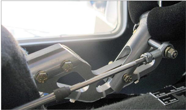
Fit the control stick to the pivot plate with an AN3-13A bolt, taking care to fit a flat nylon washer on each side between the stick and the plate. Connect the elevator cable rod end to the control stick with an AN3-21A bolt, spacer, 1/4" flat washer and a Nyloc nut as shown in the photo above and in the drawing on the next page.
