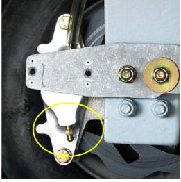
Pay careful attention to the brake fluid level in the master cylinder reservoir during this procedure and keep the fluid level topped up, otherwise you run the risk of drawing air back into the lines, which would mean starting all over again.
