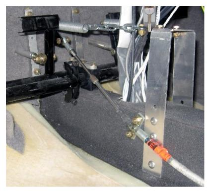
vertical. Use 3 x 7/32" TLR rivets per side as shown above.
