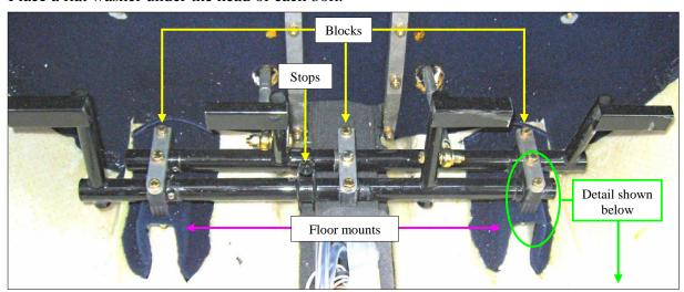
Now fit the bottom clamp plates in place inside the floor mounts one at a time: start with the front AN3-25A bolt and Nyloc nut – the front nut can be awkward to fit but if it is super glued to the plate then the plate can be held in place and the bolt can be threaded down into it.
