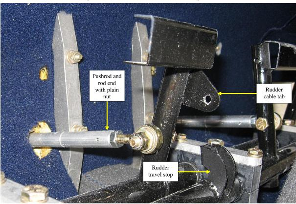
Check that the rudder pedals can move the nose wheel freely from side to side and make any fine adjustments that may be needed to have the tops of the rudder pedals all in line with the nose wheel tracking straight ahead.
