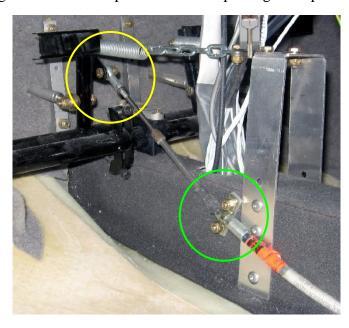
Clamp the outer cable to the console with the notched saddle clamp and backing plate and secure the clamp in place with 2 x AN3 bolts fitted from the inside of the console and Nyloc nuts with flat washers under them. Tighten the nuts to safety and mark with *TorqueSeal*.
