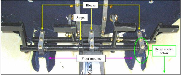
Place a flat washer under the head of each bolt.
