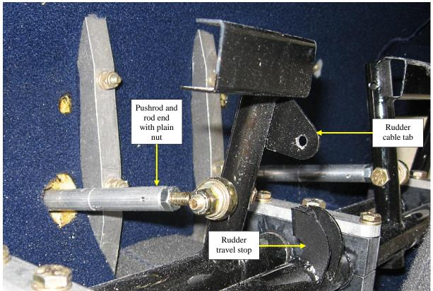
Check that the rudder pedals can move the nose wheel freely from side to side and make any fine adjustments that may be needed to have the tops of the rudder pedals all in line with the nose wheel tracking straight ahead.
