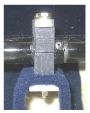
Check for free fore and aft movement of the rudder pedals.
