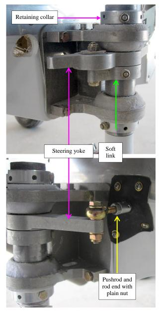
The dust cover is shown fitted in the lower photo, however it will not be final fitted until the end of this task, which is when this photo was taken.
