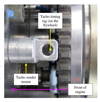
Now rotate the engine one half of a turn until the other timing tag is under the sender unit and screw the sender down until it *just* touches that tag, which should be one full turn. Back the sender unit out one half of one turn and firmly but carefully tighten the locking nut.
