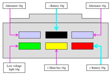
Wire the male half of a QK6 connector as shown above – note that the positive and negative wires to the battery are both 10 gauge (heavier) wire, shown above as light blue, while the rest are all 16 gauge (lighter) wire, shown above as purple.
