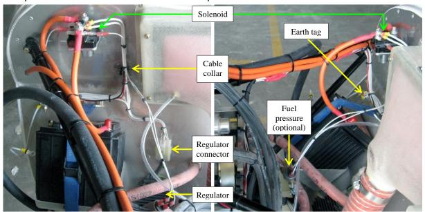
In the photos above you can see the general arrangement of the engine bay wiring.
