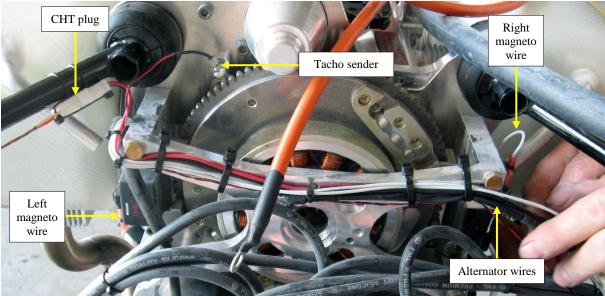
Now run the wires across the machined aluminum beam behind the flywheel as shown above. Add the alternator wire pair into the group as shown, but before you do, twist the wire pair several times so that the there are no lengths where the wire pair is straight—the full length of the alternator wires should be twisted. This will help to minimize inducing noise into the wiring harness from the alternator.
