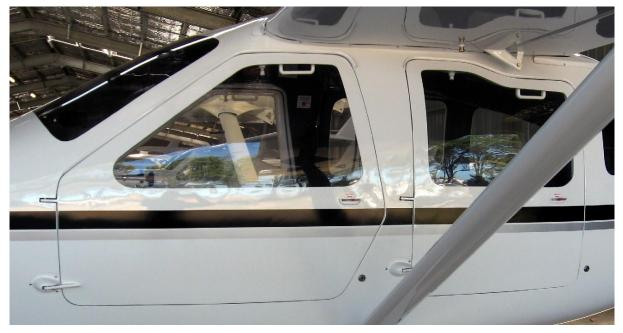
Fit each door to the fuselage. Apply a single drop of Loctite 242 to each screw, then fit the top screw first to hold the top of the door, then fit the bottom screw and check that the door closes in the centre of the door opening – there will be enough movement in the hinge screw holes to allow the door to be centred very accurately.
