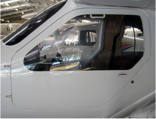
Fit each door to the fuselage. Apply a single drop of Loctite 242 to each screw, then fit the top screw first to hold the top of the door, then fit the bottom screw and check that the door closes in the centre of the door opening – there will be enough movement in the hinge screw holes to allow the door to be centred very accurately.
