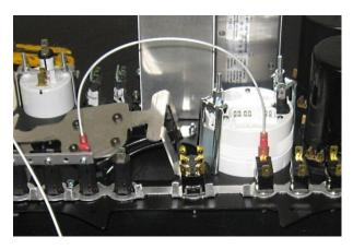
off, slip another red tag on and crimp another red female spade connector in place and heat shrink the tag on.
