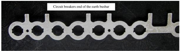
Prepare the circuit breakers and switches earth busbar by filing a 6mm notch on each side of each circuit breaker hole in order to clear the circuit breaker attachment clips as shown above.
