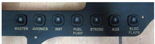
Fit the circuit breakers to the panel from the front – check the etched labels on the panel and the circuit diagram and fit the correct value circuit breaker to each hole. Press each circuit breaker in until the attachment clips click into place. Standard panel shown above.
