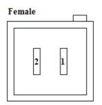
Group the wires for each plug together and trim each group to an even length, then strip 4mm from the insulation of each wire and fit the appropriate connector type to each wire: *male* spade connectors for a *female* connector body and *female* spade connectors for a *male* connector body. References to *male* or *female* will mean the connector body.
