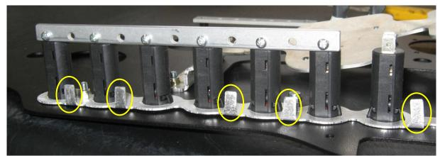
Bolt the main busbar across the lower side of the bottom contacts on the 5 and 10 amp circuit breakers only using the M3 silver screws and Nyloc nuts as shown above. Tighten firmly only: these screws and nuts are very small so take care not to over-tighten them. Note that the main busbar does **not** connect to the *Master* 15 amp circuit breaker. Fit the black "U" shaped safety bracket between the Mag switches. Now the Avionics busbar can be fitted.
