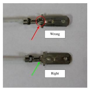
wire stops at the end of the crimp area of the connector, as indicated by the green arrow.
