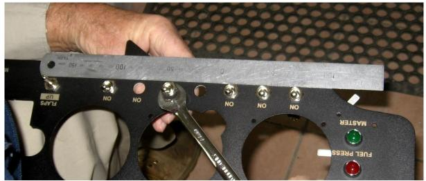
Lay a metal ruler along the bottom flats of the front retaining nuts as shown above and gently adjust each nut until all the flats are in line, then use a spanner to tighten the rear nuts firmly. Recheck each switch for alignment and make any final adjustments that may be needed.
