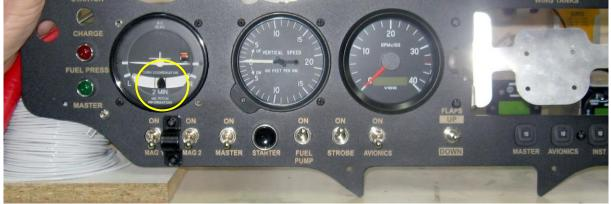
At this time the 2 points at the bottom of the panel should be placed on a known level surface and the balance ball (circled above) should be checked to see if it is in the centre.
