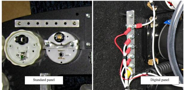
For a Standard panel the avionics busbar is located behind the "No Smoking" label above the engine instrumentation, see photo at left above – hold the busbar against the front of the panel and carefully mark and drill through the hole in each end of the busbar, first positioning the busbar so that the screw holes will not obscure the labelling.
