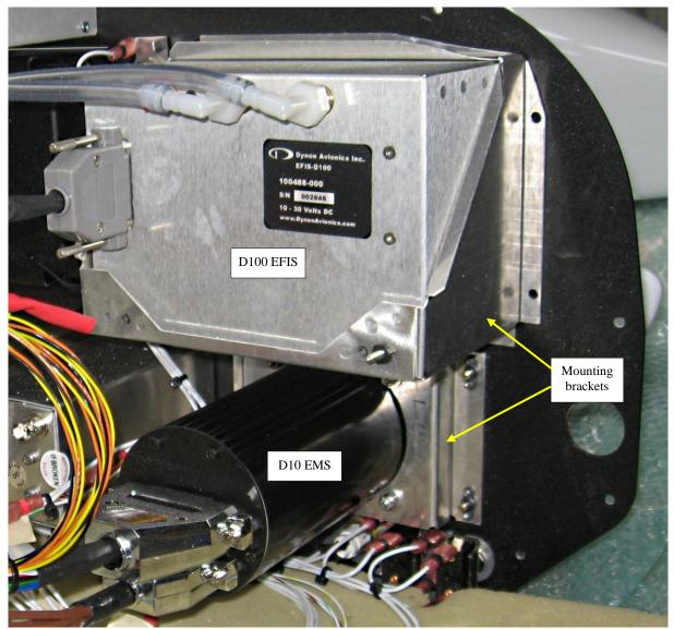
The photo above shows a *Dynon* D100 EFIS (top) and a D10 EMS (bottom) fitted to a Jumbo panel. Note the mounting brackets (arrowed) that attach each instrument to the panel.
