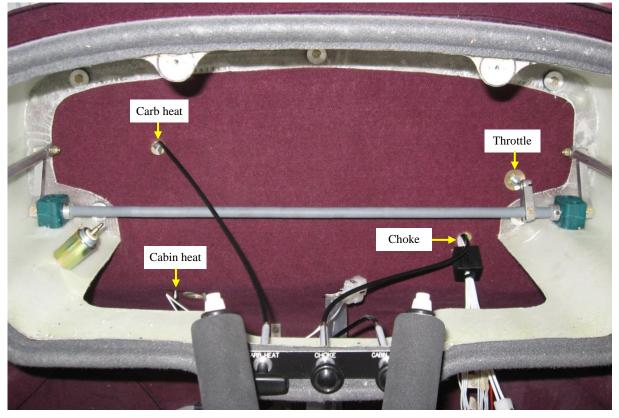
Fit the Carb Heat, Choke and the optional Cabin Heat cables to the lower centre of the instrument panel through the nameplate and secure each to the panel with a serrated washer and lock nut and then route the cables through the firewall as shown above.
