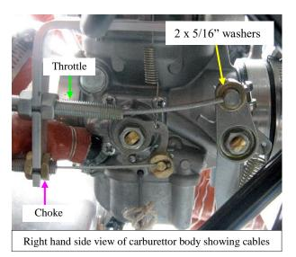
Make sure that the choke drive arm is fully forward and slip the brass ferrule over the inner cable then fit the ferrule into the hole in the drive arm. Bend the inner cable at right angles in front of the ferrule. Cut the excess inner cable off. Slip the ferrule through the retaining collar and fit to the to the drive arm with a washer and split pin fitted to the brass ferrule on the underside of the drive arm. Refer the photos and drawing on the next page for detail.
