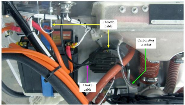
Note the cable routing shown above - this photo was taken looking straight down.
