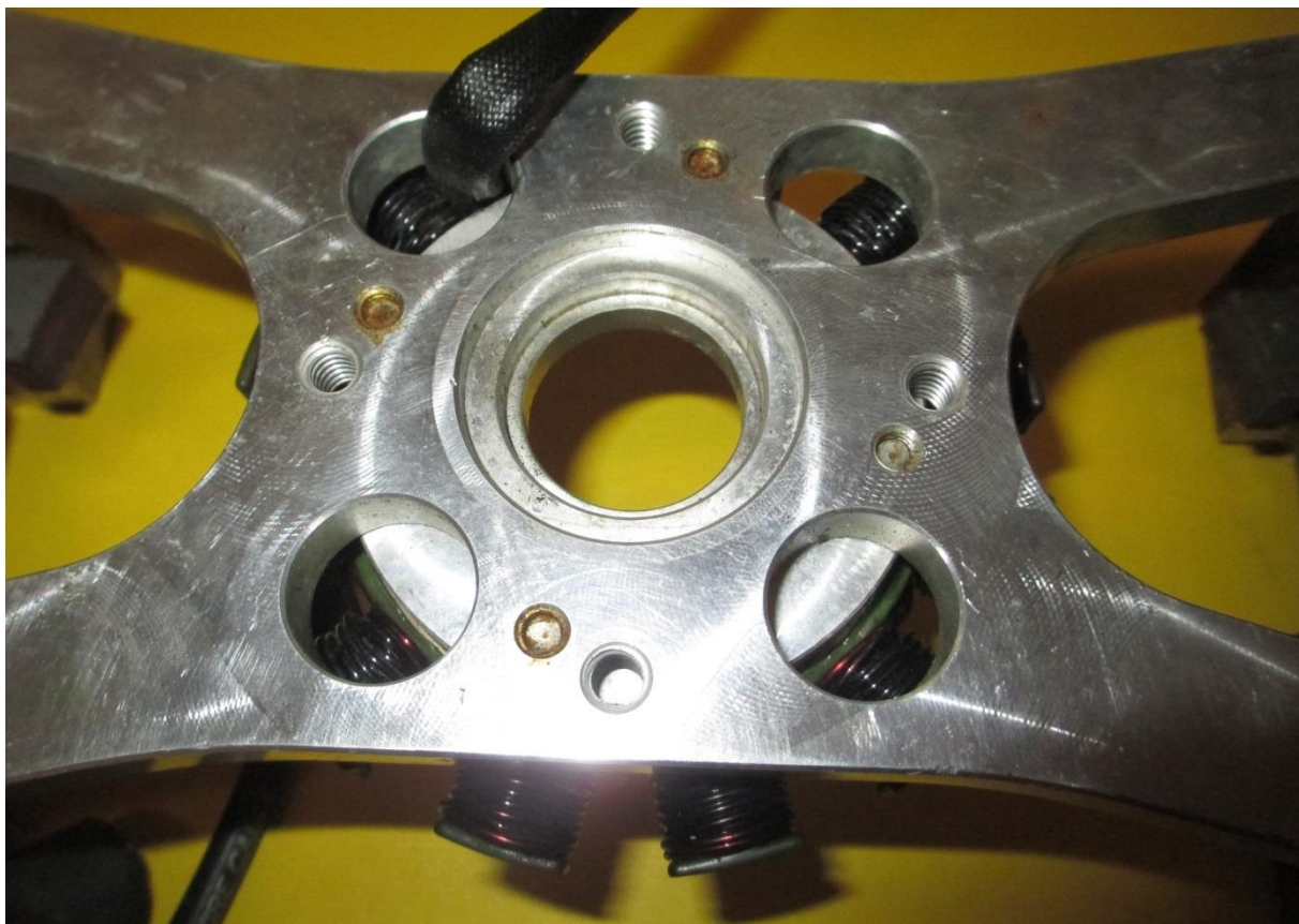
Figure 2 - Back of overheated Alternator Stator
