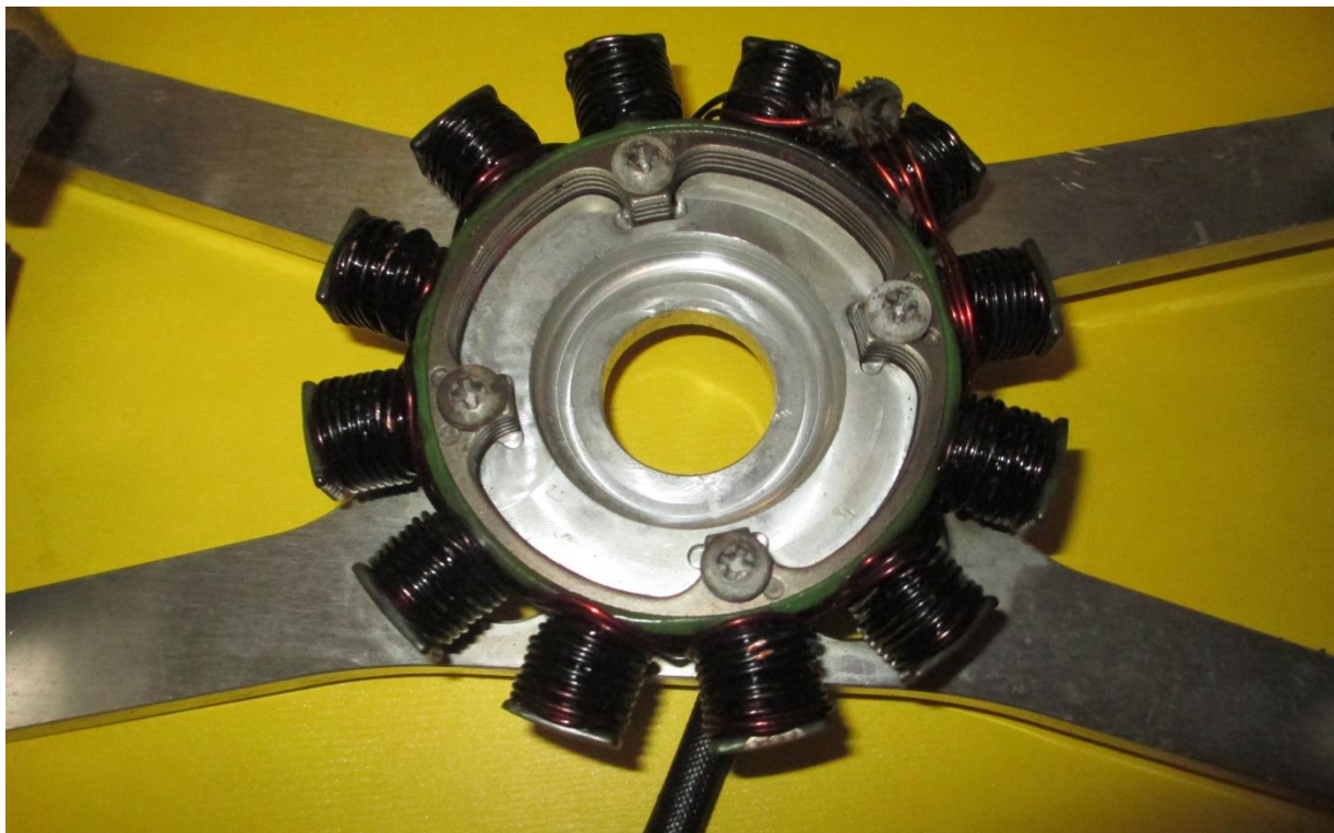
Figure 1 – Inside overheated Alternator stator (not visible when shrouded by the alternator magnet ring)
