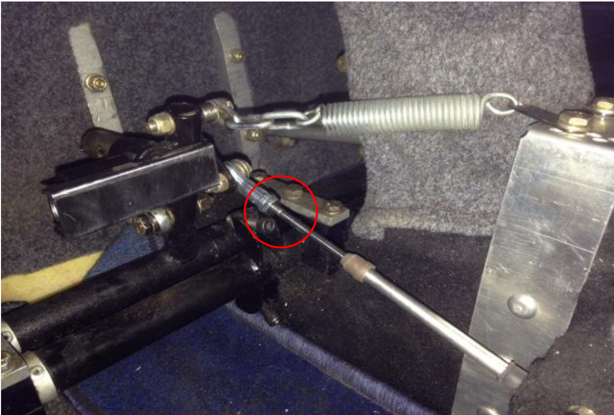
Figure 1 – Location where cable broke.
