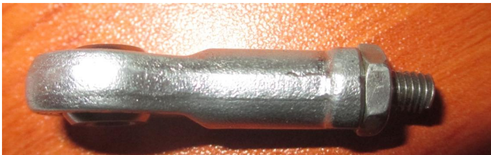
Figure 2: Rod end with broken end of cable.
