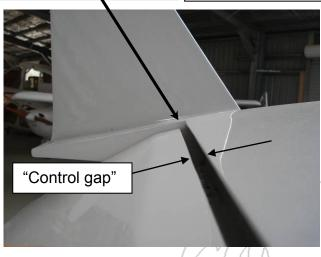
Figure 3 – Aileron Clearance
