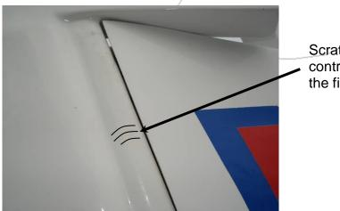
Figure 6 - Scratches on Rudder
