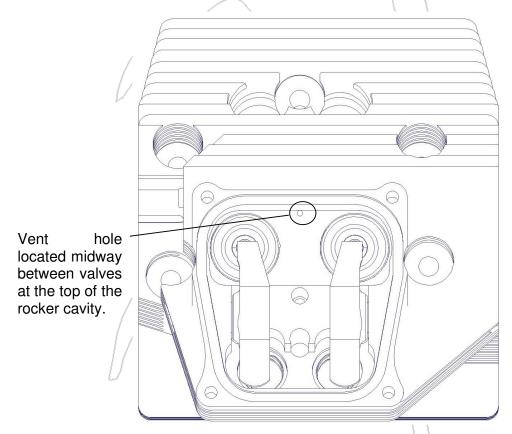
Figure 1. Vent Position – View Looking Parallel to Valves
