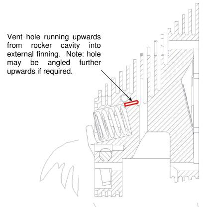
Figure 2. Sectioned View of Head Assembly - Hole Shown.
