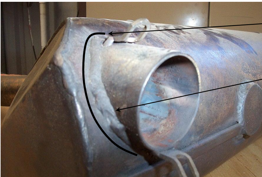
Figure 4. Example MIG-Welded Inlet Stub
