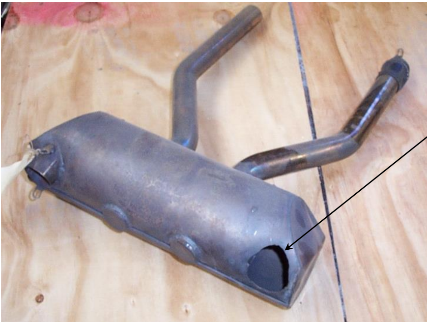
Figure 3. Typical Muffler Failure.
