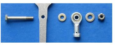
In practical terms, should a rod end fail internally in flight the rod end will still remain connected to the drive bolt and the control will continue to function.
