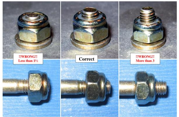
This is considered **critical** for load-bearing bolts and good practise for all other bolts. Any less than 1½ threads showing beyond the end of the lock nut means a risk of the nut not locking correctly while any more than 3 threads showing beyond the end of the lock nut could mean that the lock nut is bottoming on the thread and there is a risk overstressing the bolt and nut and/or not gripping the joined material correctly. Examples of each case are shown above.
