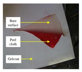
Peel cloth is typically red in colour as shown, although other colours are sometimes used. If you are in any doubt about the area that you intend to glass to, sand away the gelcoat and if you see anything that is *not* bare fibreglass then do **not** glass to it until it **is** bare fibreglass.
