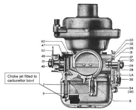
Figure 1 – Choke Schematic
