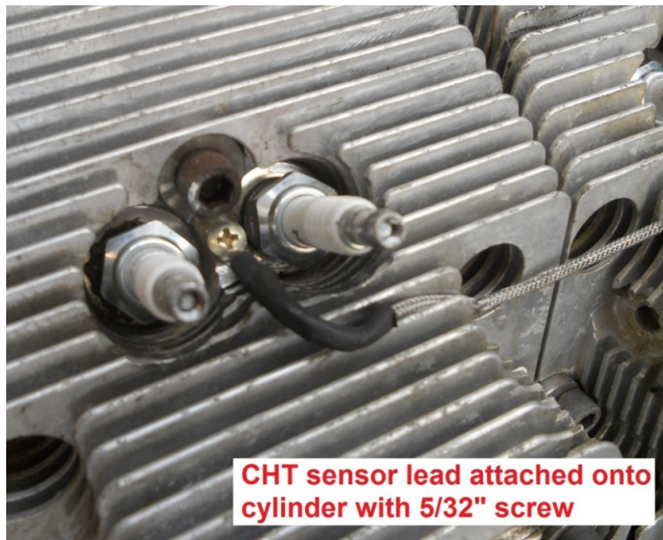
Figure 4 – CHT Cable Routing
