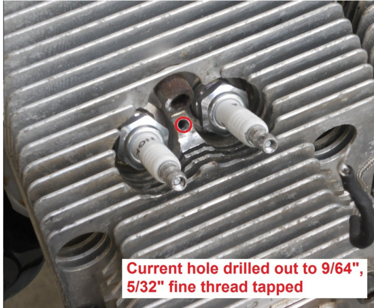
Figure 2 – Hole Tapping
